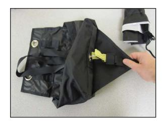
2. Inside the bag, fasten the rapid link through both loops with the kill line between them. Hand tighten the rapid link, then use a wrench to go about a 1/4 turn more.
