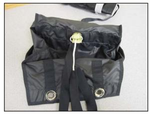
3. Holding the deployment bag from the inside, stretch the bridle taught towards the top of the triangle flap in a direction that is perpendicular from the top of the deployment bag. Introduce a small amount of slack into the bridle (1/4 inch should be fine) and bartack the bridle to the triangle flap using a stitch pattern about 1 inch in length. The idea here is to have the triangle flap load just before the bridle on deployment.
