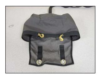
2. Install as many packing bands as necessary on the deployment bag in preparation for line stowage.
