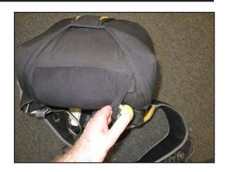
Replace the throw out pilot chute handle over top of the bridle. Verify the edge of the spandex pouch meets with the edge of the bridle cover.
