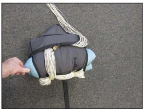
5. Stop stowing suspension lines when you have about 18 inches of line left unstowed between the risers and the deployment bag.
