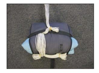
6. You should have about 18 inches of suspension line left unstowed between the risers and the deployment bag.
