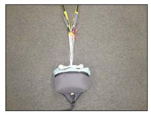
7. Stow the risers and packed parachute into the container according to the manufacturer's instructions.
