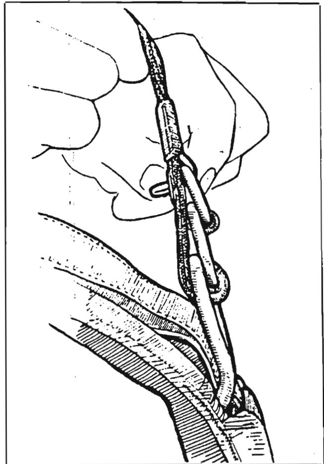
5) Continue threading the white loop through the grommet on the end of the cable housing. The flat side of the cable housing grommet should be against the riser.
