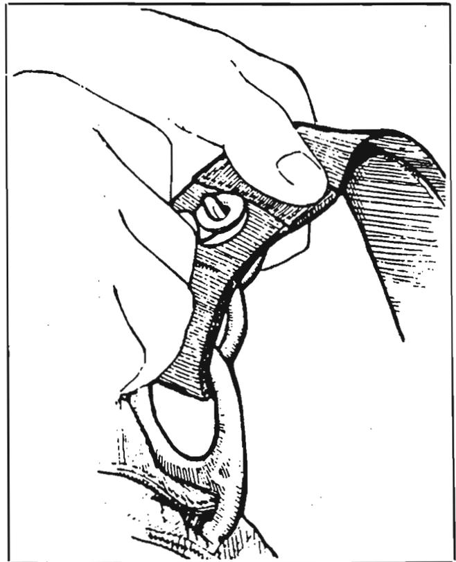
6) Thread the yellow cable through the white loop, making sure the loop isn't twisted. Be careful with the cable so you don't bend it too sharply or kink it. Insert the free end in the channel on the back of the riser.
