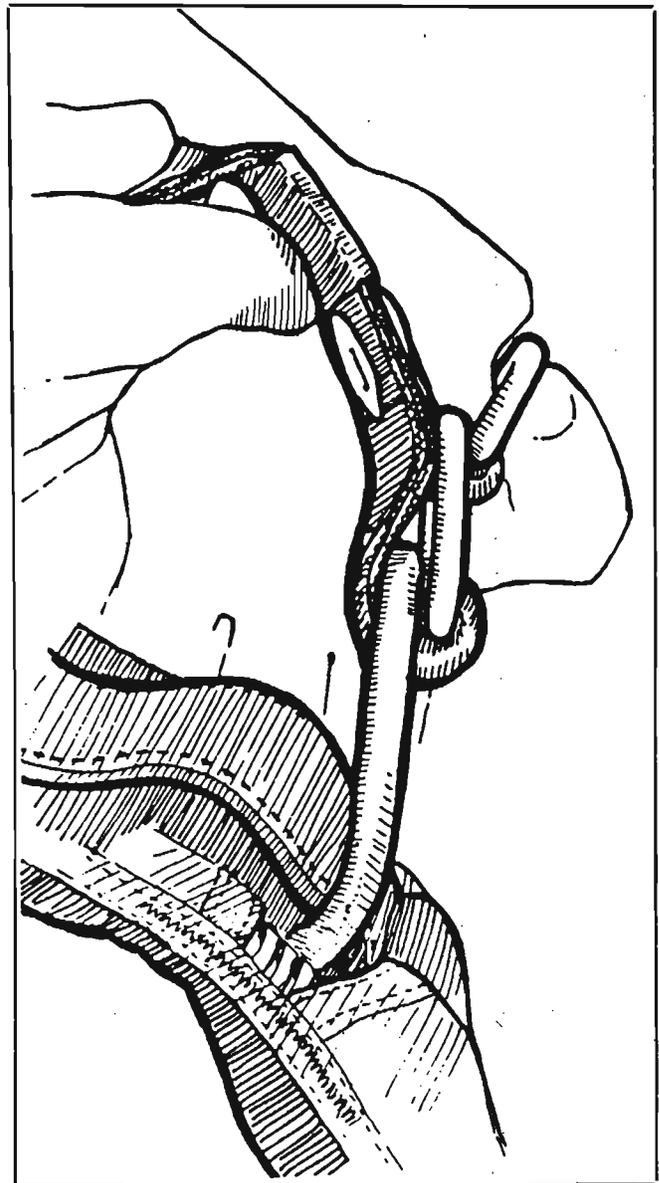
4) Bring the white loop over the small ring only and then through the riser grommet so it pokes out the back of the riser.
