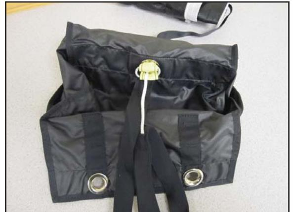
3. Holding the deployment bag from the inside, stretch the bridle taught towards the top of the triangle flap in a direction that is perpendicular from the top of the deployment bag. Introduce a small amount of slack into the bridle (¼ inch should be fine) and bartack the bridle to the triangle flap using a stitch pattern about 1 inch in length. The idea here is to have the triangle flap load just before the bridle on deployment.
