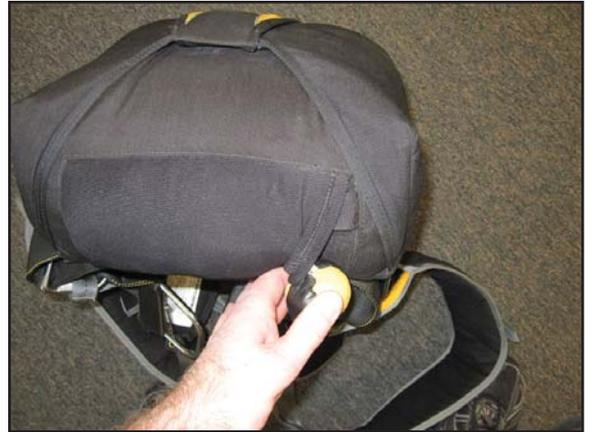
5. Replace the throw out pilot chute handle over top of the bridle. Verify the edge of the spandex pouch meets with the edge of the bridle cover.
