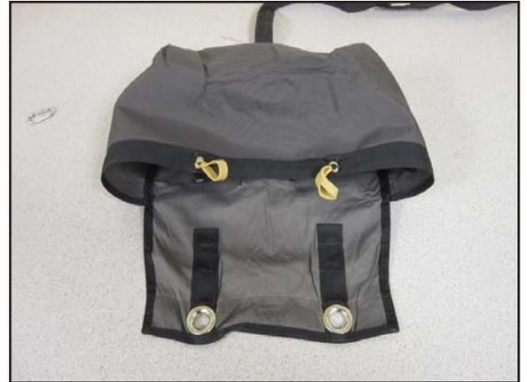
2. Install 1 additional packing band for the locking stow of the free-stow pocket.
