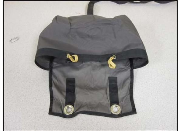
2. Install as many packing bands as necessary on the deployment bag in preparation for line stowage.
