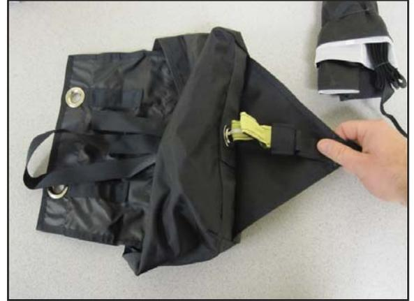
2. Inside the bag, fasten the rapid link through both loops with the kill line between them. Hand tighten the rapid link, then use a wrench to go about a ¼ turn more.
